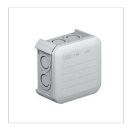
The junction boxes are made of a thermoplastic polypropylene polymer with plug-in seals made of ethylene vinyl acetate (EVA). This allows installation of cables either directly through the 7 x Ø20 seals, or the seals can be cut with a knife at the pre-marked points, in order to create an insertion opening for cables or pipes. Alternatively, cable glands can be pushed through the openings instead of the seals and locked with a locknut from the inside.
