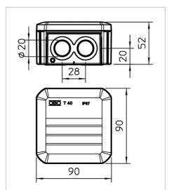
Standard version: flame-resistant, testing temperature 650  $^{\circ}\text{C}.$ F version: highly flame-resistant, testing temperature 960 °C.
