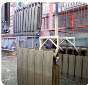
Cooling the fins in water after oven process
