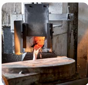
Raw aluminium being melted at the start of process
