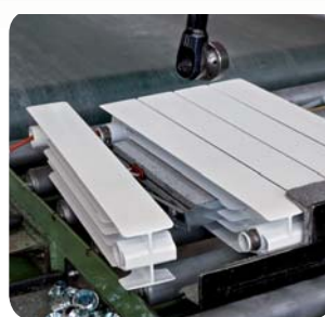
Unique silicone joint between fins
