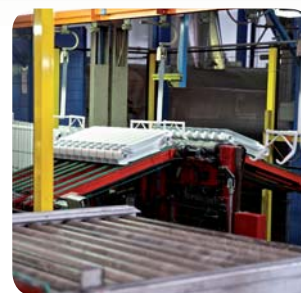
Radiators on way for pressure testing and quality control
